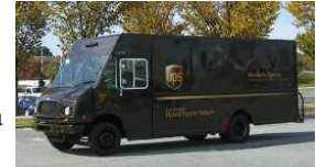
FCCC truck with Eaton drive billed as 'world's first hydraulic hybrid delivery vehicle'
