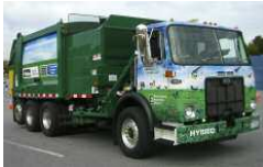
Autocar refuse truck with Parker hydraulic drive
